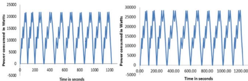
Fig. 18.19 Power consumption of the proposed SEV for a gradient of 10.2° (left) and 15° (right)
