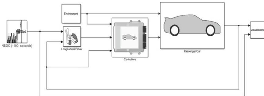
**Fig. 18.20** Electric vehicle reference application from MATLAB/Simulink
