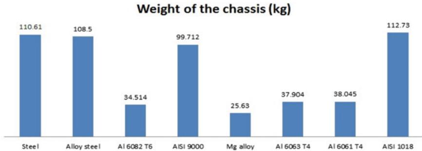
**Fig. 18.6** Chassis weight comparison for purpose-built SEV
