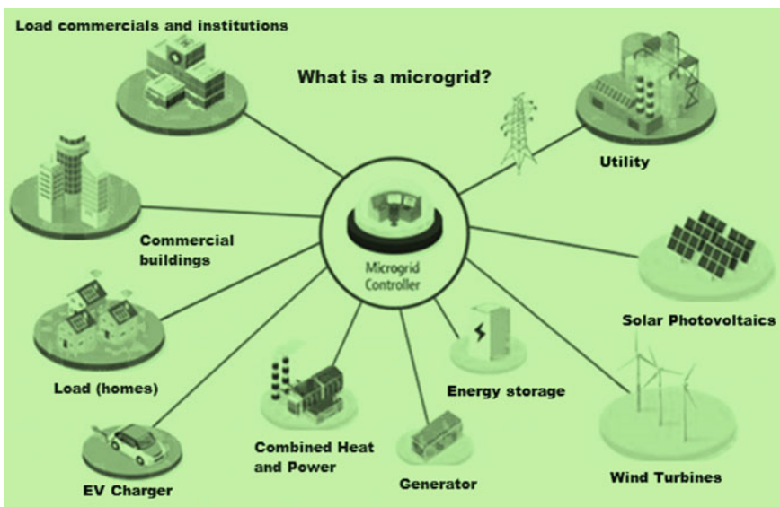
Fig. 17.2 Structure of microgrid
