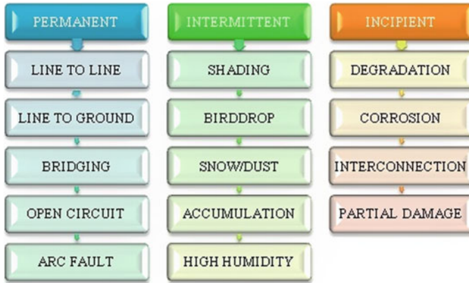
Fig. 3.3 Types of faults in PV Array
