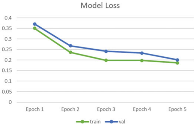
Fig. 9 Training versus validation loss for VGG-16 finely tuned architecture
