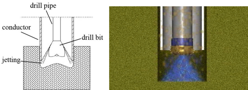
Fig. 4. The model of jet drilling
