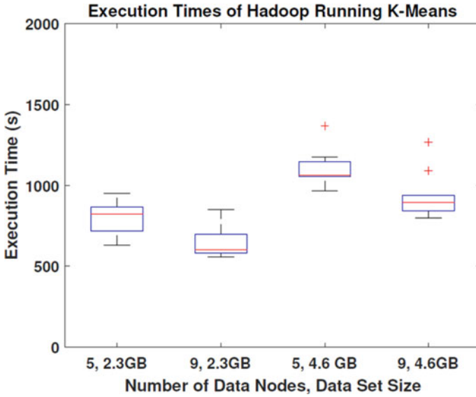
Fig. 8 Execution times of the k-means experiments with the 40 million row data set as the cluster size changes. Included also are the execution times for the same node configuration for the original experiment
