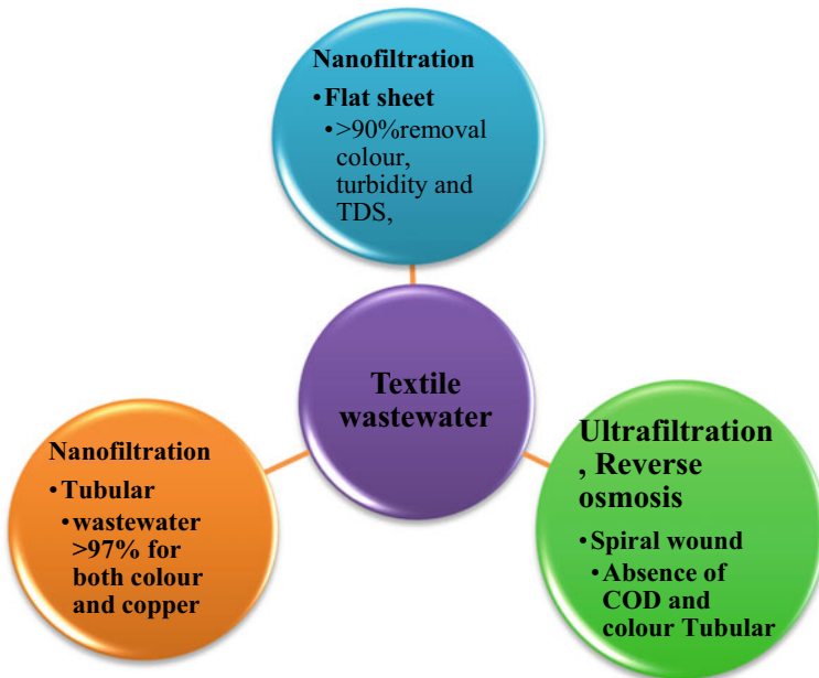
Fig. 5 Illustrations of membrane use for textile wastewater treatment. Symbols COD—carbon organic dissolved; TDS—total dissolved solids
