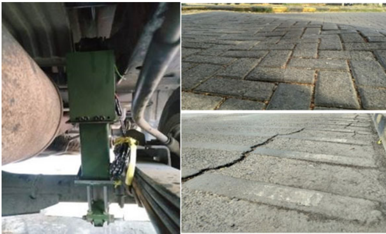
Fig. 4. RESA installation in vehicle suspension, road bump and speed trap
