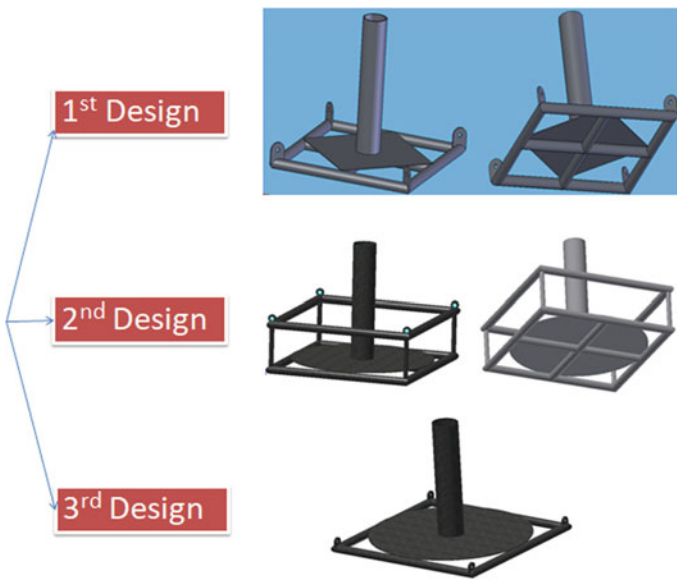
Fig. 2. Design models of the BOP transport skid
