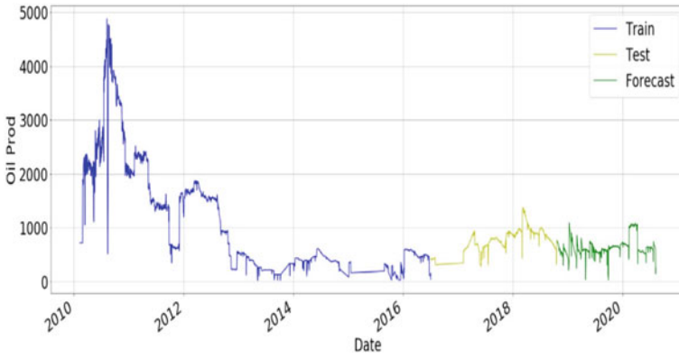
Fig. 19 Application of RNN + LSTM to forecast well-3 oil production
