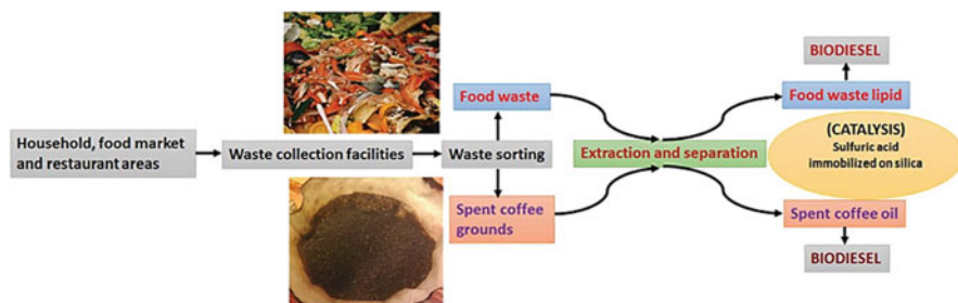
Fig. 4.5 Biodiesel production from food wastes. (Adapted from Karmee 2017)
