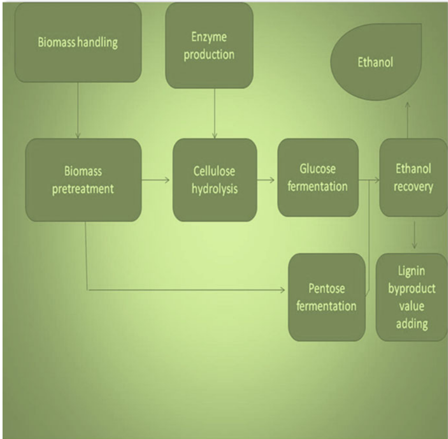
Fig. 9.3 Flow diagram for the production of bioethanol
