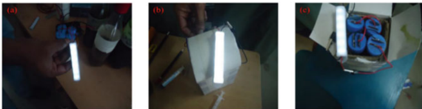
Fig. 2 a An experimental set up for myrobalan cell. b An experimental set up for lemon cell. c An experimental set up for tomato cell
