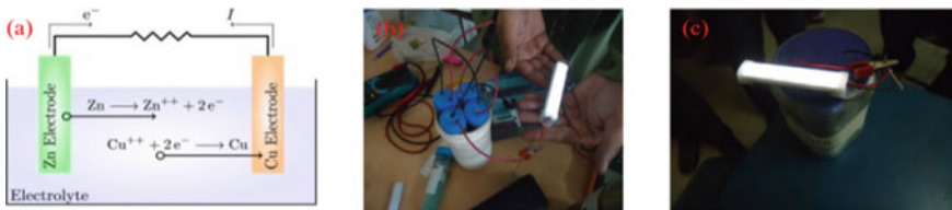
Fig. 1 a Experimental technique of chemical reaction. b An experimental set up for PKL cell. c An experimental set up for aloe vera cell
