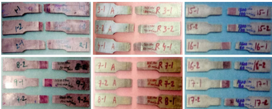
Fig. 6 Few tensile specimens after tensile test
