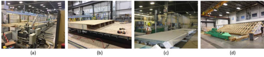
Fig. 1 Typical factory-based home construction facility: a Wall framing station, b Floor station, c Wall sheathing station, and d Roof production station [3]
