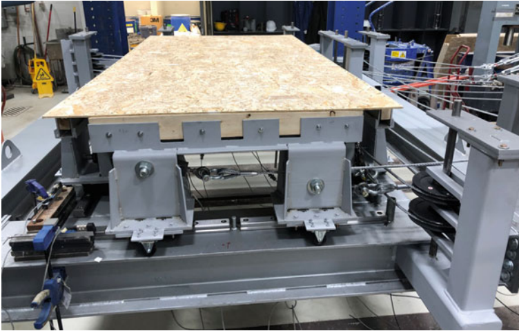
Fig. 3 Test setup for 6.4 mm OSB sheathing panel with 63.5 mm nail @ 50 mm
