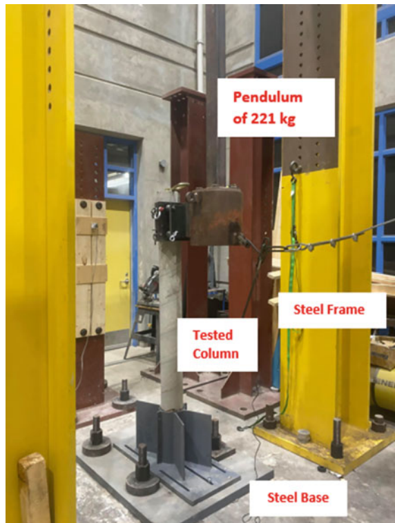
Fig. 1 Test set-up of lateral impact test using pendulum machine
