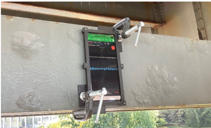
Fig. 1 Vibration testing set-up used for eyebars vibration testing. Smart phone display shows the g-force meter under nominal conditions (no forced excitation)
