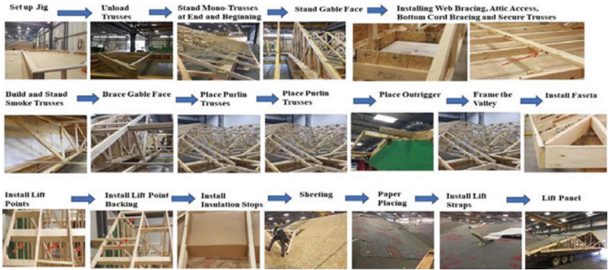
Fig. 2 Work breakdown of current roof module production process [3]
