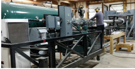
Fig. 2 Large bore FOD gun at UNB BAM Lab
