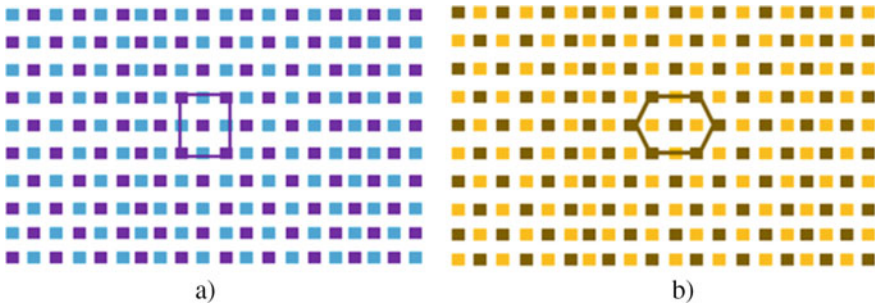
Fig. 3 a Rectangular grid, b simulated alternate hexagonal grid
