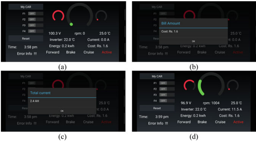
Fig. 3 Screenshot of android application: a dashboard, b electricity costing, c battery consumption, d motor speed
