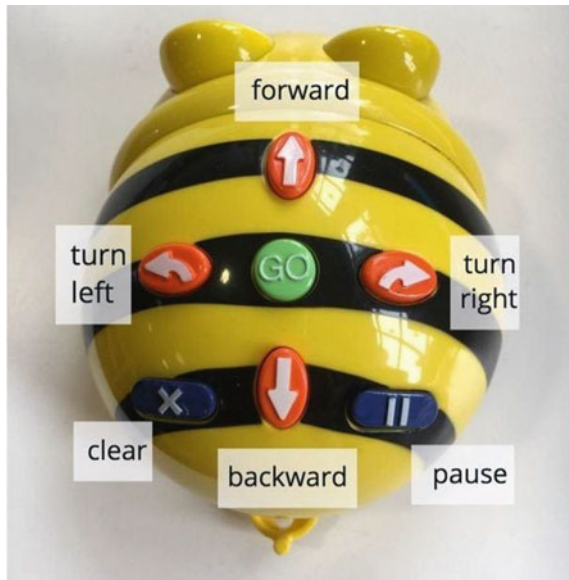
Fig. 22.2 The structure and controls of a Beebot
