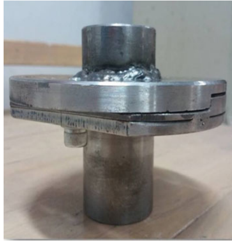
Image 7 Side View of asymmetrical chuck
