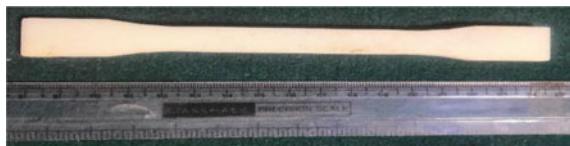
Fig. 3 3D printed flat tensile pattern
