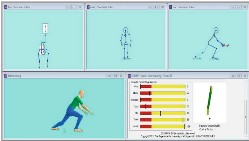
Fig. 2 Picture of data for ergonomic analysis entered in 3D SSP software
