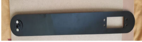
Fig. 3 The link after getting laser cut
