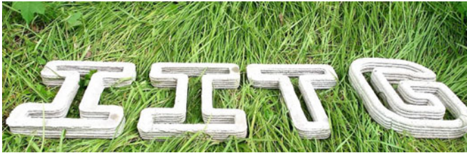
Fig. 6 3D concrete printed letters of IITG
