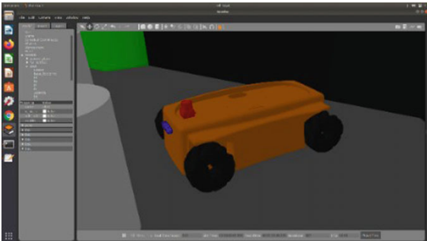
Fig. 5 LiDAR Sensor mounted on robot
