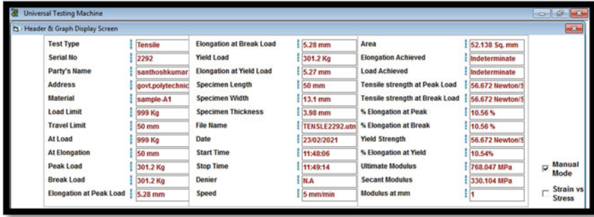
Fig. 5 UTM test results screen of a sample printed in flat orientation with 20 mm/s print speed
