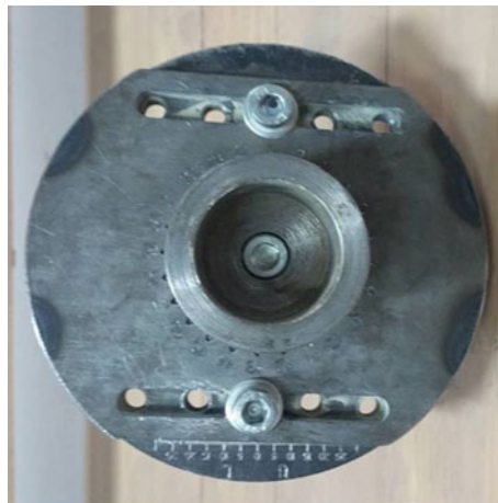
Image 6 Top View of asymmetrical chuck
