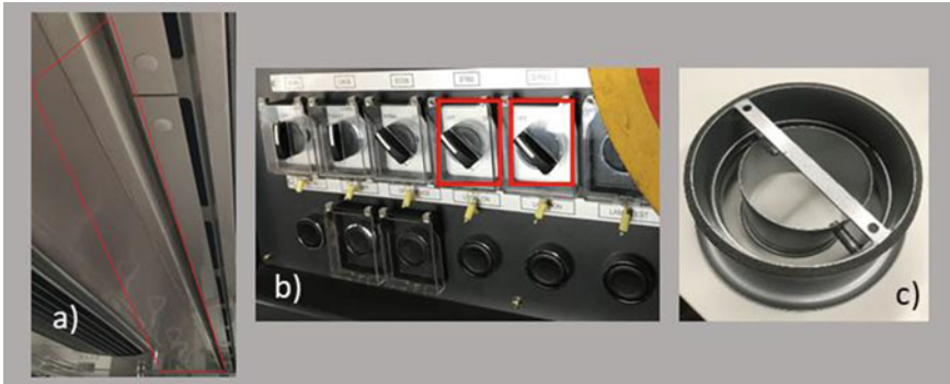
Fig. 3 Parts examined for case study— a Part 1: diffuser ceiling moulding (1.5–2 m); b Part 2: control switches; c Part 3: air-conditioning nozzle
