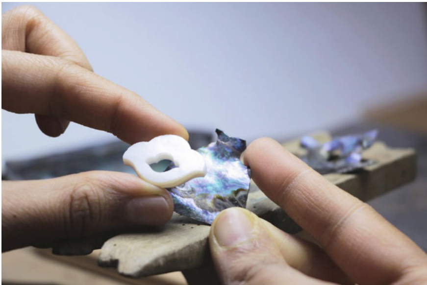
Fig. 4 Simple motif being prepared for inlay during manufacturing
