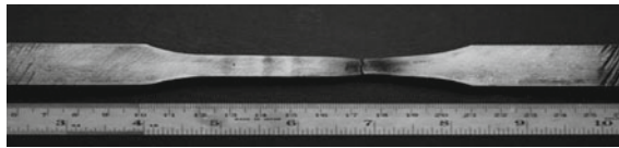
Fig. 7 Sand cast specimen after tensile testing
