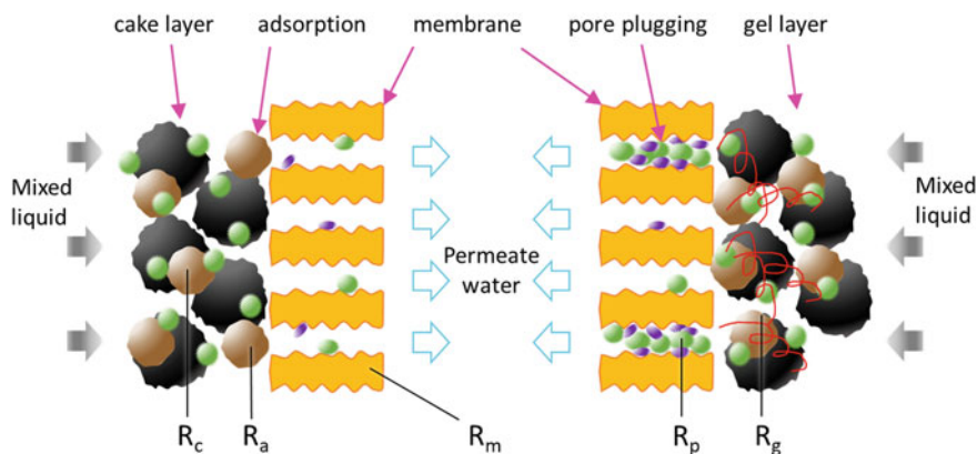
Fig. 4 Types of membrane fouling and the resulting resistances ( R_a , resistance to adsorption; R_c , resistance of cake layer; R_g , resistance of gel layer; R_m , resistance of membrane; and R_p , resistance of pore plugging)
