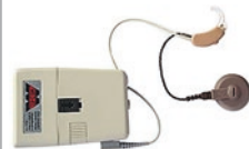
Speech processor featuring an ear-level microphone—1989
