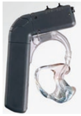
World's first DUET speech processor having hearing aid component to amplify low-frequency sound signals—2005
