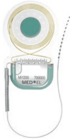
SYNCHRONY CI with MRI compatible implant magnet—2014
