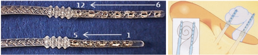
Fig. 3.7 SPLIT electrode with two branches. The short branch has five channels to be placed in the upper basal turn stimulating the low frequencies and the long branch with seven channels to be placed in the lower basal turn stimulating high frequencies
