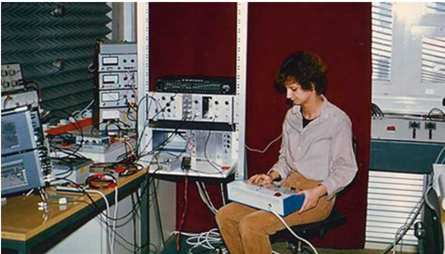
Fig. 3.11 Mini-suitcase-sized investigational audio processor
