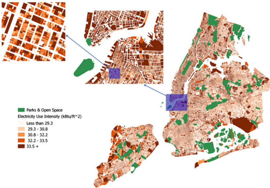
Fig. 2 The map of New York City with the predicted electric energy use intensity for each property (Kontokosta and Tull 2017)
