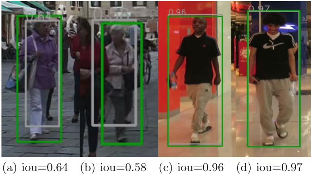
Fig. 4. Process of collecting training samples. The green bounding box is the groundtruth. The gray bounding box is generated by the detector and the tracker, with the iou of the two bounding boxes as the score.
