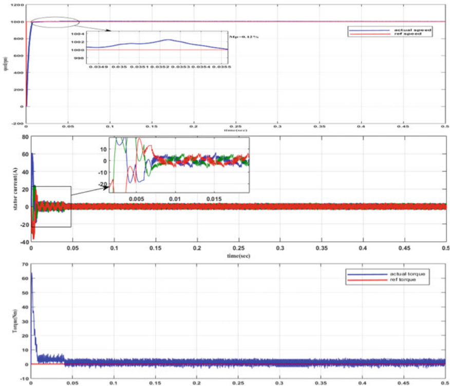
Fig. 6 MOGA-based PID speed controller PMSM drive: starting characteristics
