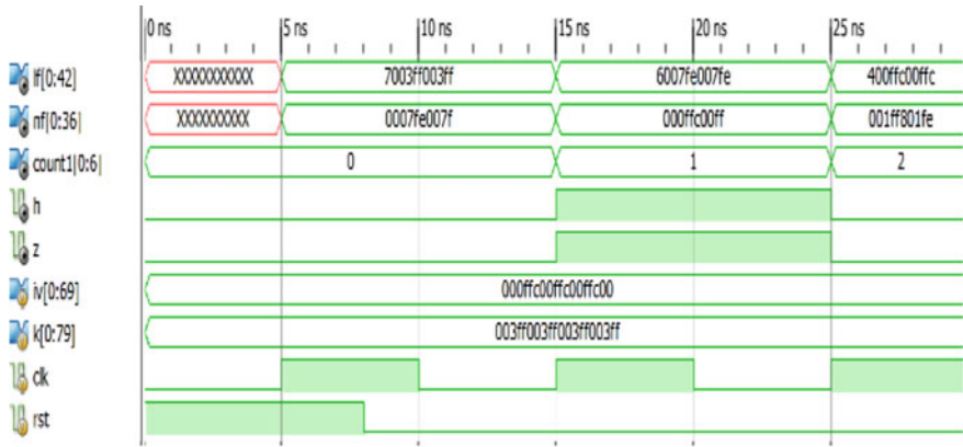
Fig. 5 Simulation output for initialization phase of Fruit-80
