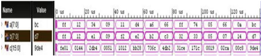
Fig. 6 Simulation results of 8-bit Vedic multiplier using MAMR architecture
