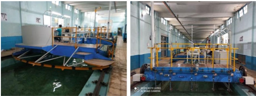
Fig.1 Current Meter Rating Trolley (CMRT) facility at CWPRS
