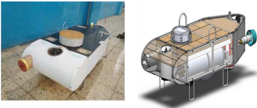
Fig. 2 Schematic view of coral reef monitoring robot (CBOT)
