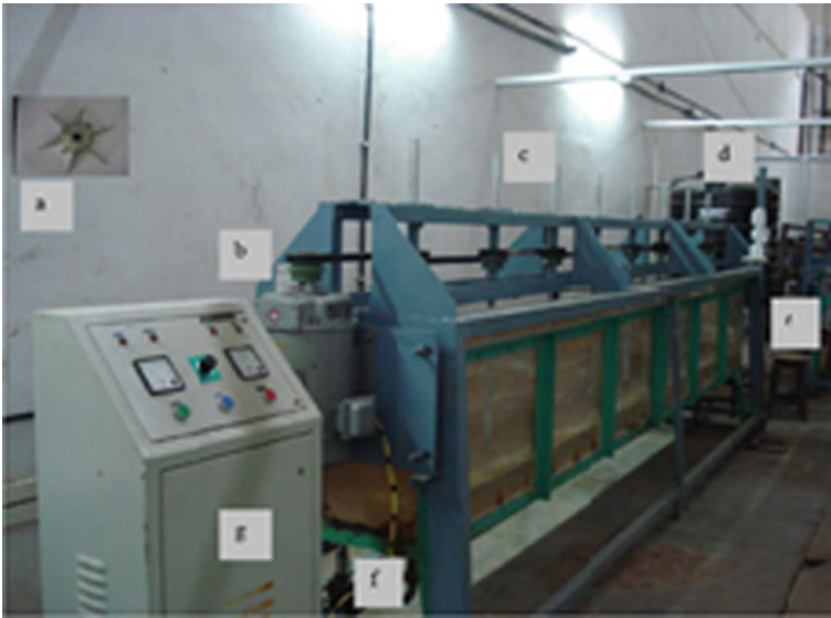
Fig. 1 Experimental system (a-impeller, b-DC motor, c-impeller placing, d-storage tank, e-ADV, f-recirculating pump and g-display control panel)
