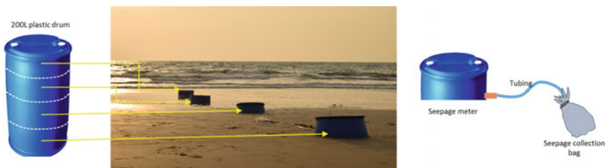
Fig. 2 Seepage meter design and deployment in the intertidal zone
