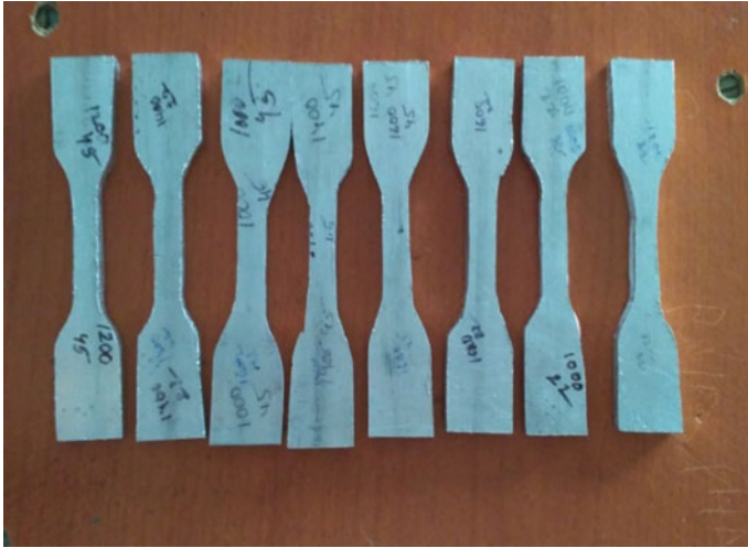
Fig. 6 Specimens for tensile test (ASTM-E8)
