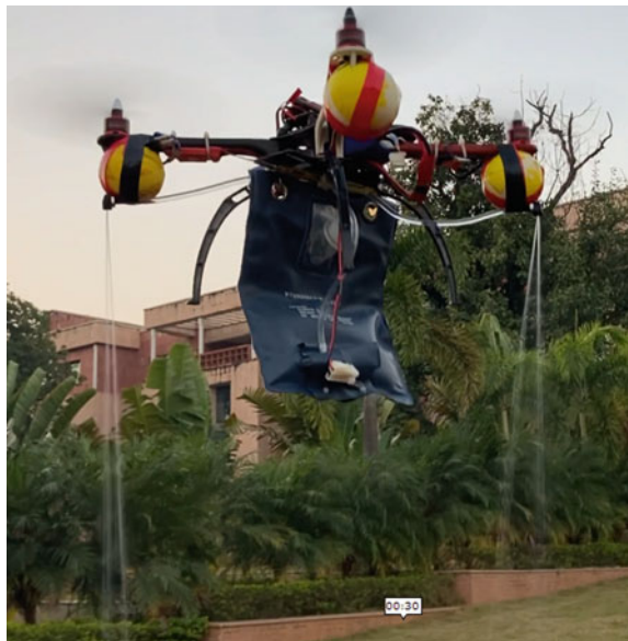
Fig. 3 Quadcopter spraying pesticide over the plants
