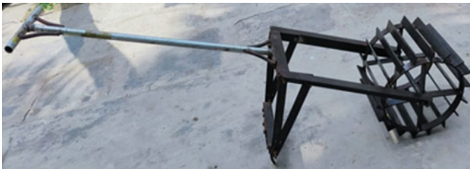
Fig. 7 Manually operated weeder
