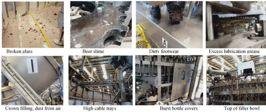
Fig. 3 Dirt sources identified and removed in Step 2 of the AM
