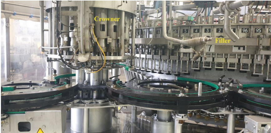
Fig. 2 The glass bottle is filled and crowned
