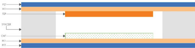
Fig. 2 Sectional working of CNF-FEP-based TENG. Author’s image
