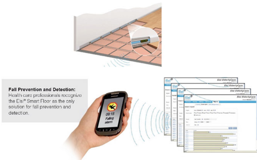
Fig. 5 System operation of Elsi® Smart floor [9]
