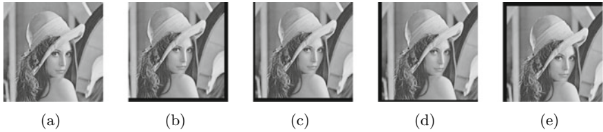
Fig. 2 a Original Lena image, b shifted Lena image by (-20, -20) , c shifted Lena image by (-20, 10) , d shifted Lena image by (-10, -10) , e shifted Lena image by (20, 20)
