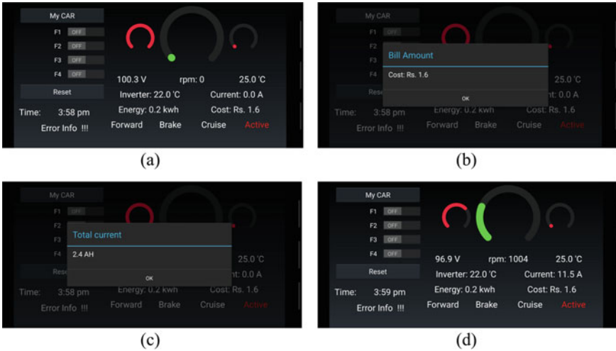
Fig. 4 Screenshot of android application: a Dashboard, b electricity costing, c battery consumption, d motor speed
