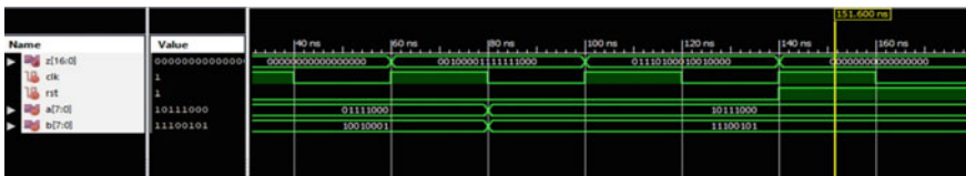
Fig. 10 Simulation result for implementation 1: A and B are the 8-bit inputs. Clk signal controls the incoming values and output results of the MAC unit. Reset signal is used to reset the accumulator
