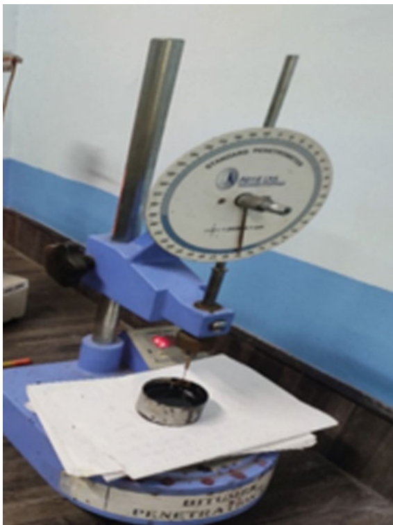
Fig. 2 Bitumen penetration test
