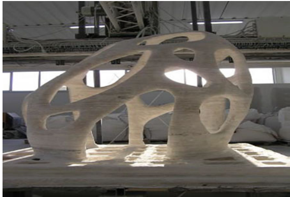
Fig. 3 D-shape 3D printed structure [12]
