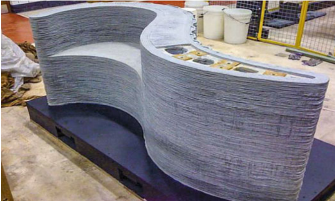
Fig. 7 Concrete printing created a full-scale bench with usable voids and post-tensioned reinforcing [21]
