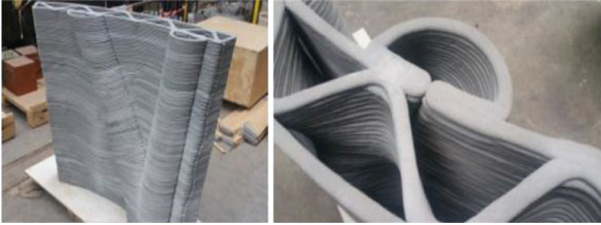
Fig. 8 Multifunctional wall element [21]
