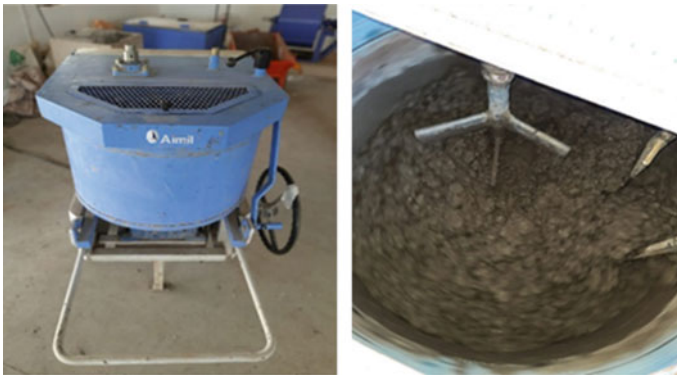
Fig. 2 Pan mixer and mixing process
