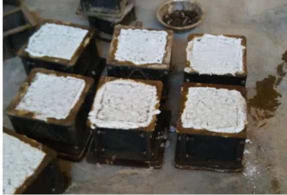
Fig. 2 Concrete cubes with high activator ( \text{Na}_2\text{SO}_4 ) dosage
