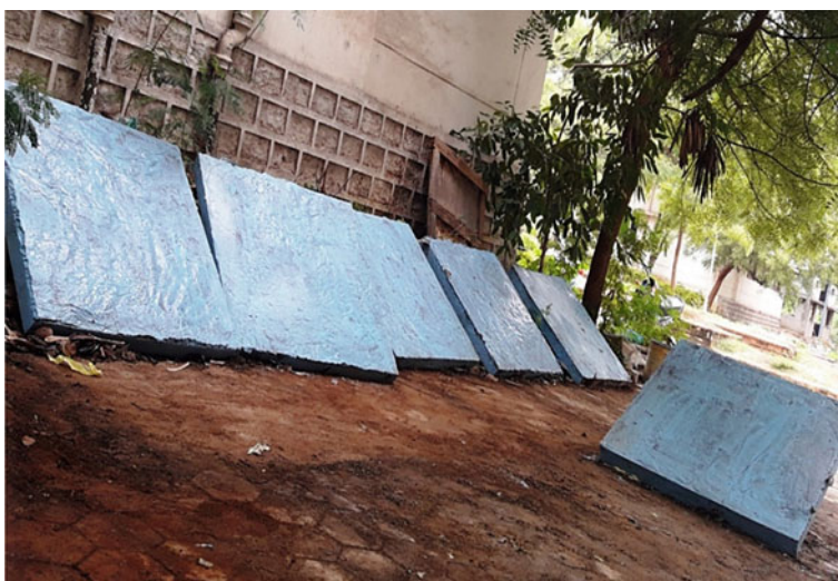
Fig. 6 Slab specimens after 28 days curing
