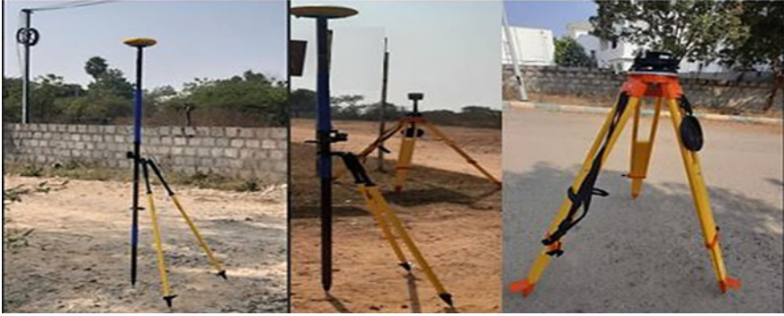
Fig. 2 DGPS survey equipment used in the field
