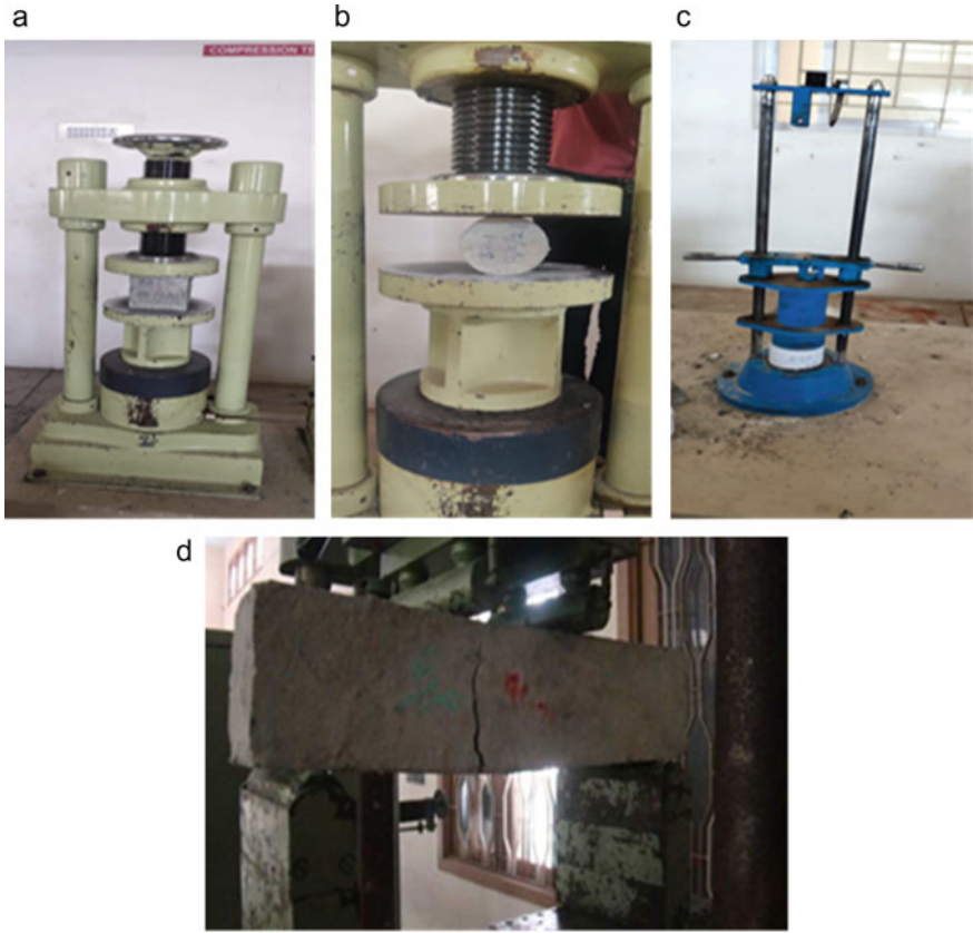
Fig. 3 a-d Test setup for compression, split tension, impact, and flexural tension
