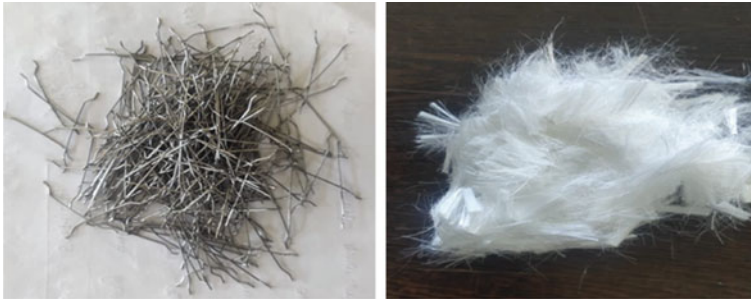
Fig. 1 Steel and polyester fibers
