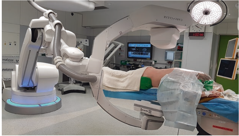
Fig. 37.1 The Artis zeego imaging system (Siemens) during intraoperative use. Image originally published by Pireau et al. [50]. Republished with permission by Springer Nature
