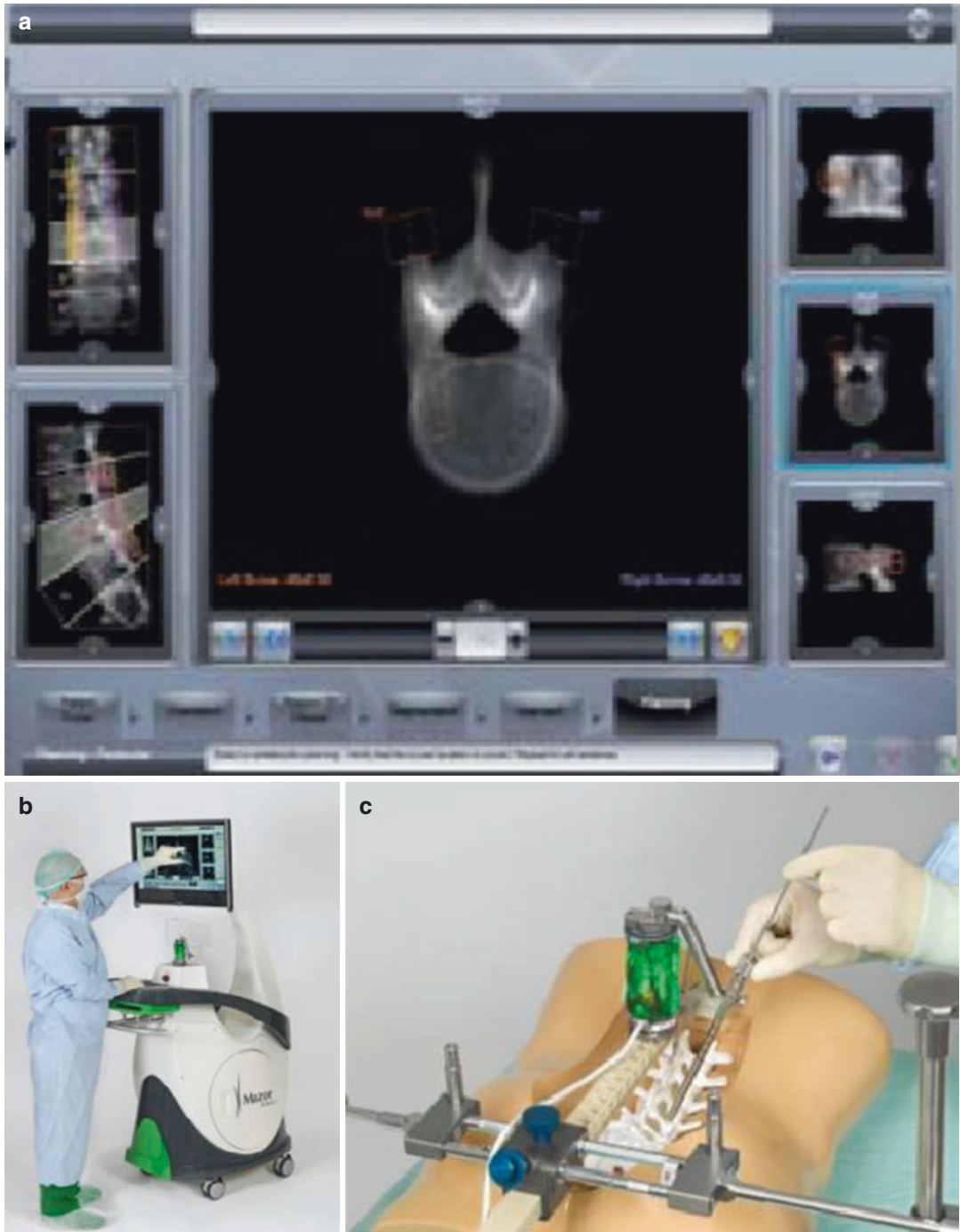
Fig. 25.3 Renaissance is a second-generation robotic system for spine surgery developed by Mazor Robotic Inc. (Caesarea, Israel). Renaissance consists of three components. (a) CT-based 3D planning software, (b) Workstation, and (c) Miniature robot
