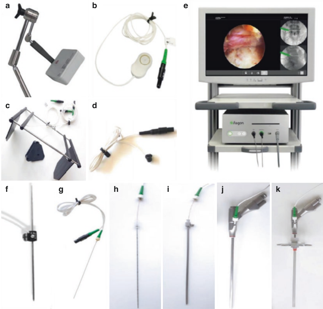
Fig. 15.1 Instrument of EM-based navigation system for lumbar foraminoplasty. (a) magnetic field generator, (b) MultiPad, (c) MaperBrige, (d) Localizer, (e) computer mainframe and monitor, (f) Kirschner wire, (g)
