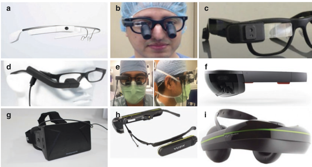
Fig. 33.17 Multiple examples of HMD-devices used for augmented-reality applications: (a, b)—Google Glass; (c)—Optinvent; (d, e)—Vufine; (f)—Microsoft HoloLens; (g)—Oculus Rift; (h)—Vuzix M300; (i)—Vuzix iWear. Images in A (Google Glass), F (Microsoft HoloLens), and
