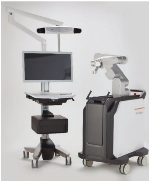
Fig. 25.4 The CUVIS-spine system (Curexo Inc. Republic of Korea) allows surgical instruments and screws to be inserted into the planned path generated by a surgeon using intraoperatively scanned 2D or 3D images. The main console and robotic arm make a trajectory for the insertion of the screw
