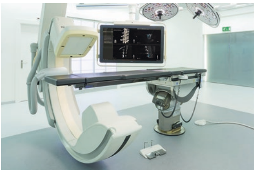
Fig. 33.12 OR setup of the augmented-reality surgical navigation system (ClarifEye) with 4 patient-tracking cameras integrated into the C-arm. The AR view is presented on the monitor. Photo courtesy of Philips Healthcare
