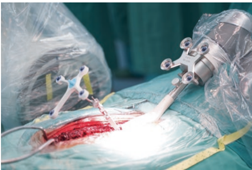
Fig. 27.1 TiRobotic-assisted screw placement system
