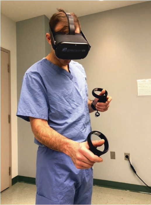
Fig. 42.1 A surgical trainee using a contemporary immersive virtual reality simulator. The hardware is comprised of the Oculus Quest system, complete with head-mounted display and hand-based controllers. The software is produced by Precision OS Technology (Vancouver, Canada)
