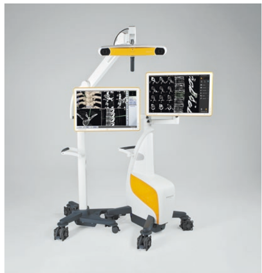
Fig. 1.3 Intraoperative infrared camera, computer, and monitor (Curve®, Brainlab). The infrared camera tracks reflective material placed on surgical instruments as well as a reference array rigidly affixed to the patient. The computer and associated software create 3-D projections depicting the surgical instruments relative to the patient’s intraoperatively acquired anatomy. Image copyright owned by Brainlab, used with permission
