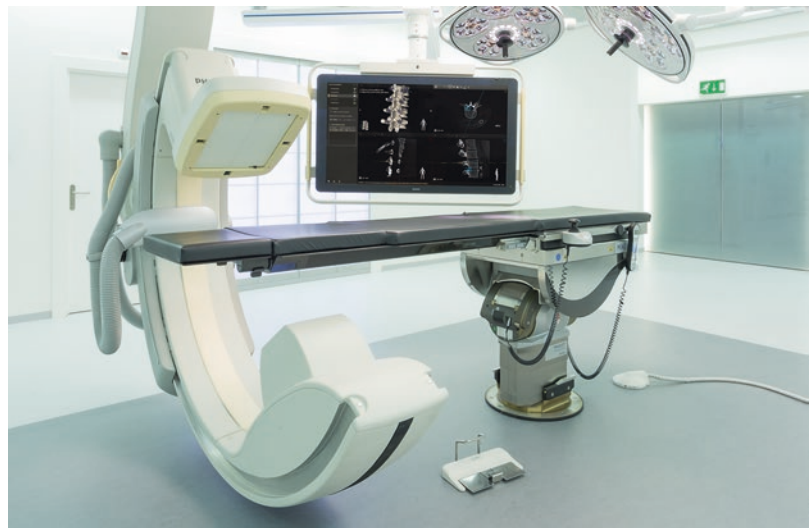
Fig. 38.1 OR setup of the augmented reality surgical navigation system (ClariEye) with four patient tracking cameras integrated into the C-arm. The AR view is presented on the monitor. Photo courtesy of Philips Healthcare
