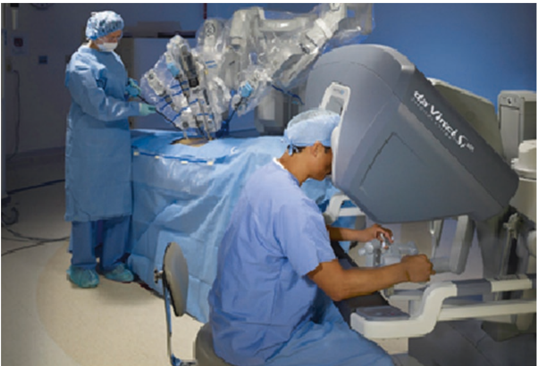
Fig. 25.2 da Vinci Surgical System (Intuitive Surgical, Sunnyvale, CA). The da Vinci is a system where the operator controls the device at a station away from the operatory room
