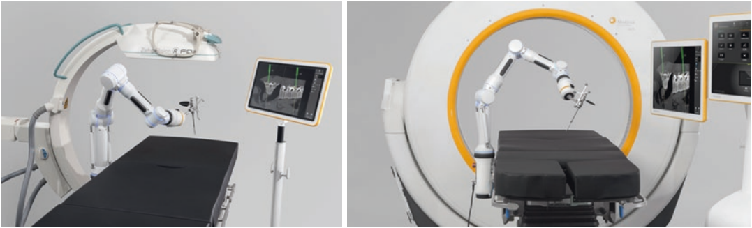
Fig. 1.5 Example of intraoperative setup integrating robotic arm with intraoperative imaging. Left panel: Ziehm© cone beam CT and Cirq© Brainlab robotic arm affixed to surgical table. Right panel: robotic arm affixed
