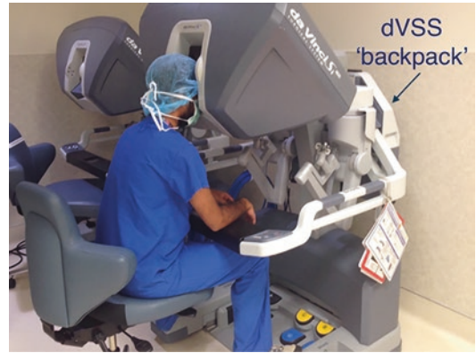
Fig. 39.5 The da Vinci surgical console with the da Vinci Skills Simulator (dVSS) attached. Image courtesy of dVSS, Intuitive Surgical, Sunnyvale, USA and originally published by Bric et al. [19]. Republished with permission by Springer Nature
