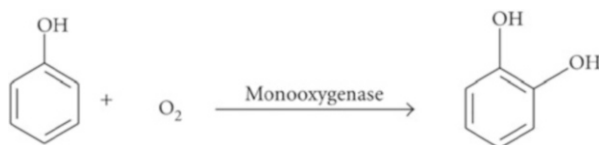
Fig. 1 Degradation of phenol by monooxygenase (Arora et al., 2010)
