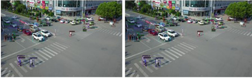
Fig. 4 Detection results on VisDrone test-dev dataset. C4 configuration (left) and FPN (right)
