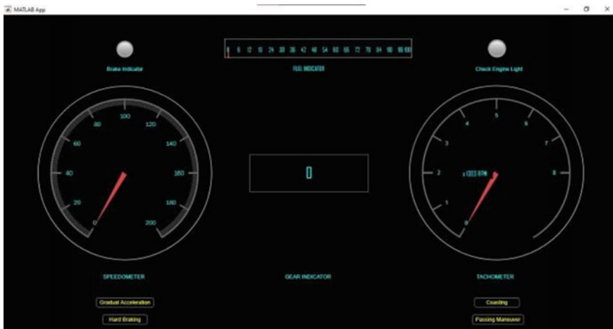
Fig. 6 Vehicle dashboard created using MATLAB's App Designer
