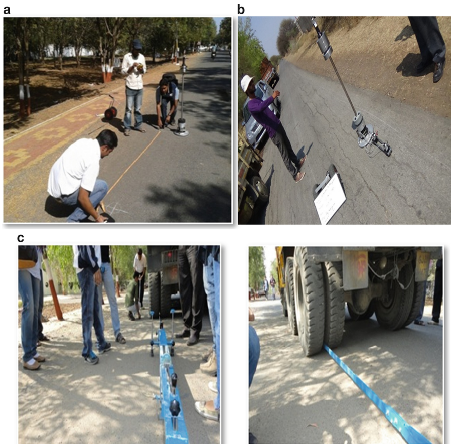
Fig. 2. (a). LWD tests points, (b). Testing of LWD, (c). BBD test on the study location.
