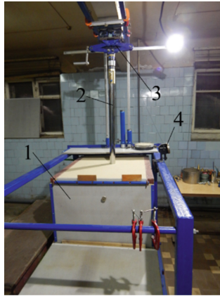
Fig. 7. Experimental system: front view. 1 – soil box; 2 – model pile; 3 – mechanical jack; 4 – displacement gauge.
