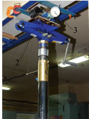
Fig. 8. Loading system. 1 – model pile; 2 – mechanical jack; 3 – dynamometer.
