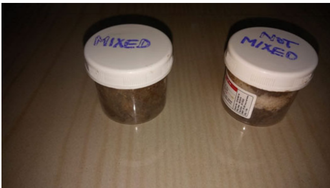
Fig. 12 Container to contain the samples for further consideration. Sample A: Not Mixed (a layer of inner diaper material is clearly visible). Sample B: Mixed (as it is thoroughly mixed with the garden soil the sample is not clearly visible)
