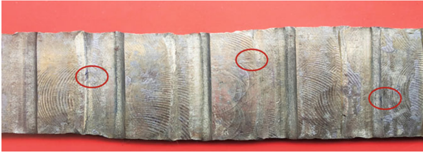
Fig. 2 Formation of micro-cracks on the constrained groove pressed ARMCO Fe sheet
