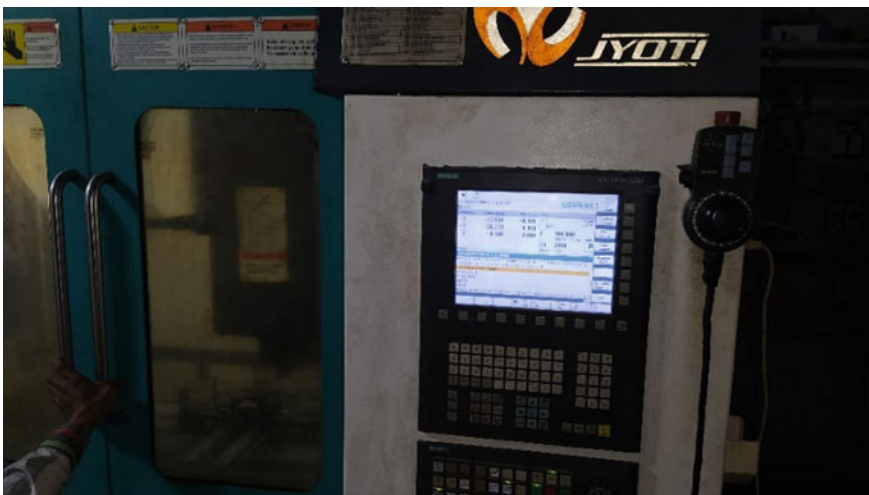
Fig. 3 Vertical machining centre—Siemens controlled-VMC 640
