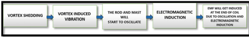
Fig. 5 Flow chart of working mechanism
