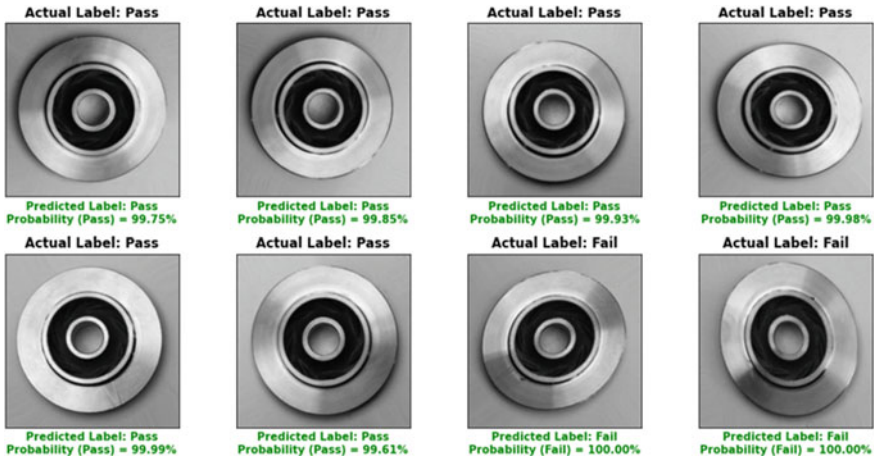
Fig. 6 Predicted samples with the actual/predicted label and the confidence score of each detection
