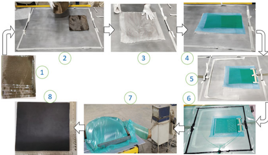
Fig. 2 Experimental setup of VARTM process with necessary steps
