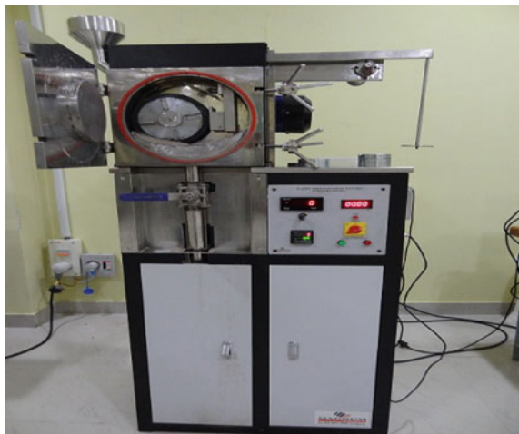
Fig. 1 Slurry abrasion test rig
