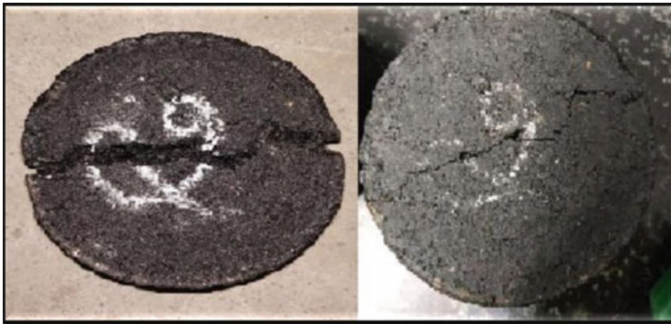
Fig. 3 Crack width before and after heating and healing cycle
