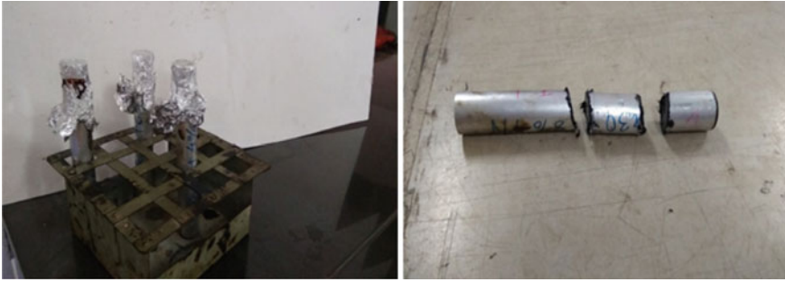
Fig. 3 Aluminum tubes used in the storage stability test
