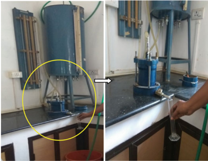
Fig. 2 Experimental setup of constant head permeability test
