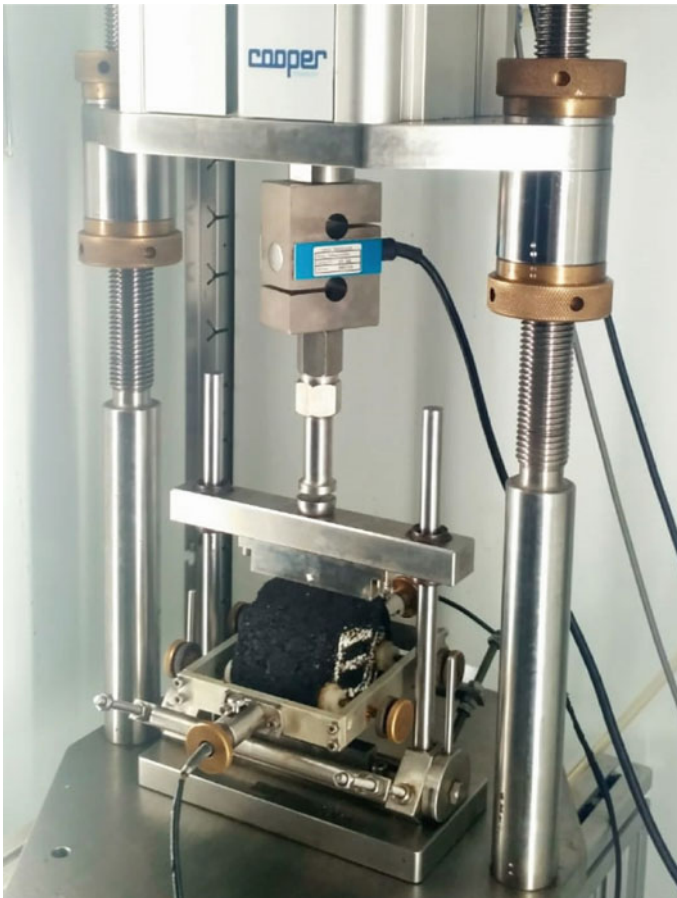
Fig. 5 Test assembly for resilient modulus test
