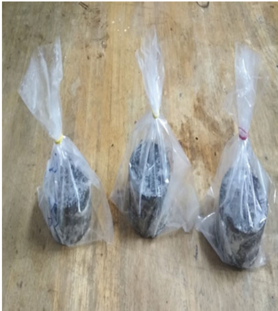
Fig. 8 Samples after freeze-thaw cycle in plastic bag
