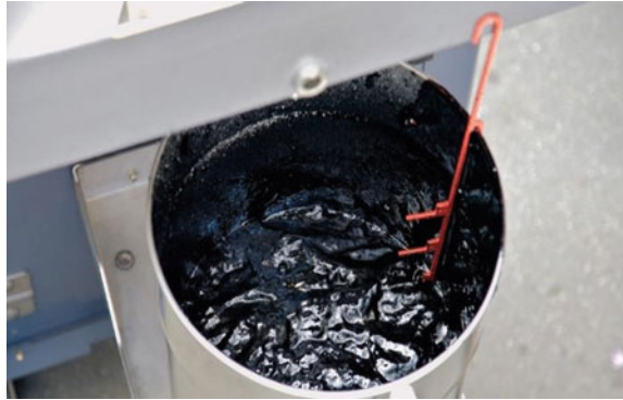
Fig. 2 Image showing foam bitumen with a dip stick (Wirtgen, 2004)
