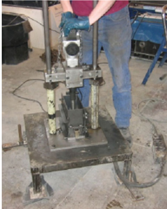
Fig. 1 Clamped-on vibrator used along with an electric hammer to replicate the industrial procedure of paver block production (Source Soutsos et al. [2])
