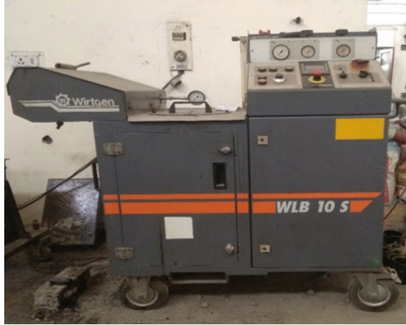
Fig. 1 Image showing the foam plant (WLB 10 S)
