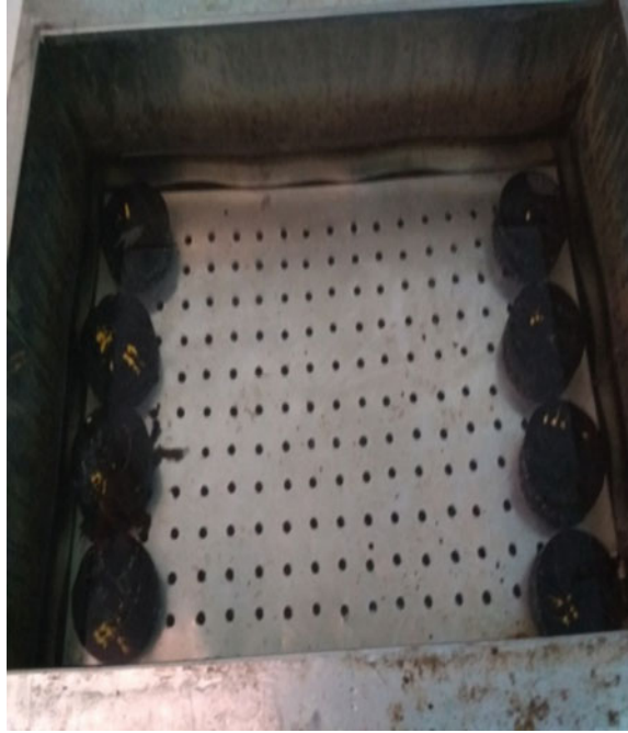
Fig. 10 Samples in water bath at 25 °C after removing from plastic bag
