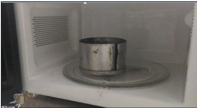
Fig. 1 Sample with aluminum mold kept in microwave oven used in present study
