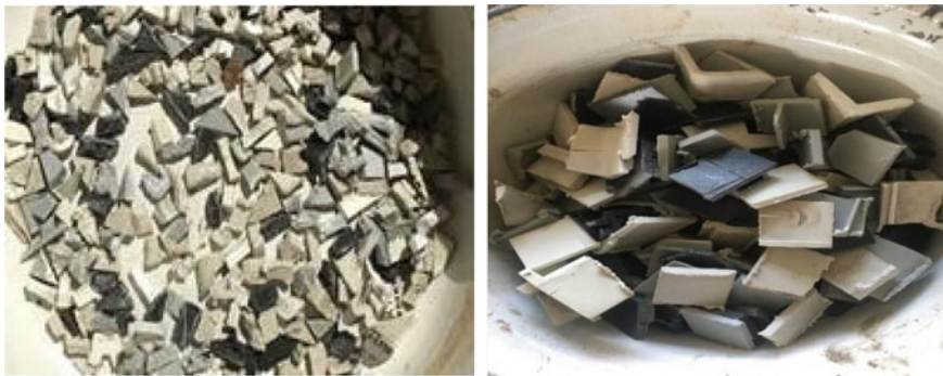
Fig. 3 Shredded E-waste plastic of size 2.36 mm and 13.2 mm (retained IS sieve)
