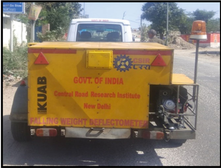
Fig. 3 View of FWD used for structural evaluation of pavement
