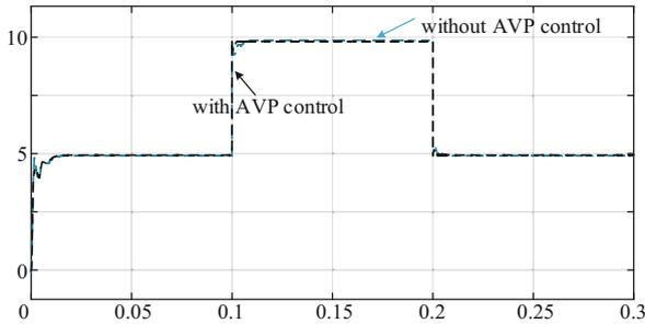
(b) output current of the converter
