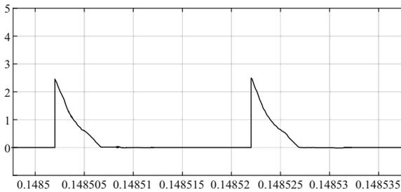
**Fig. 12.** The current of clamp diode simulation waveform
