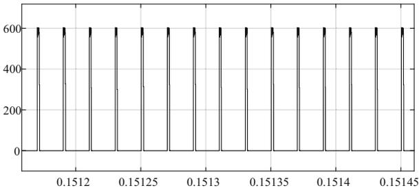
**Fig. 11.** The soft switching conditions of the main power switch
