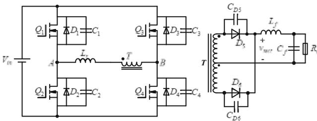
Fig. 2. Phase shifted full bridge circuit topology
