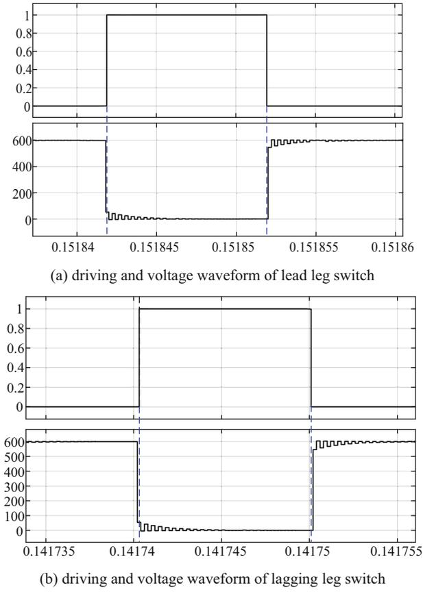
**Fig. 10.** The soft switching conditions of the main power switch
