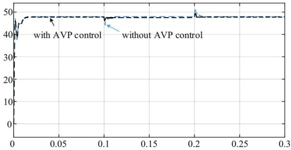
(a) output voltage of the converter
