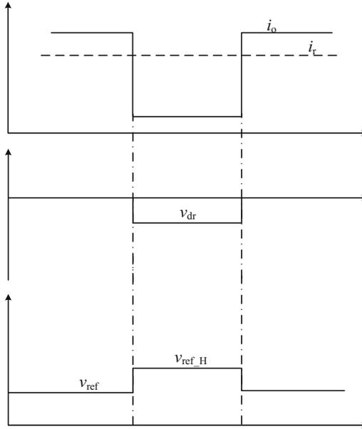
Fig. 5. Operation principle of AVP control
