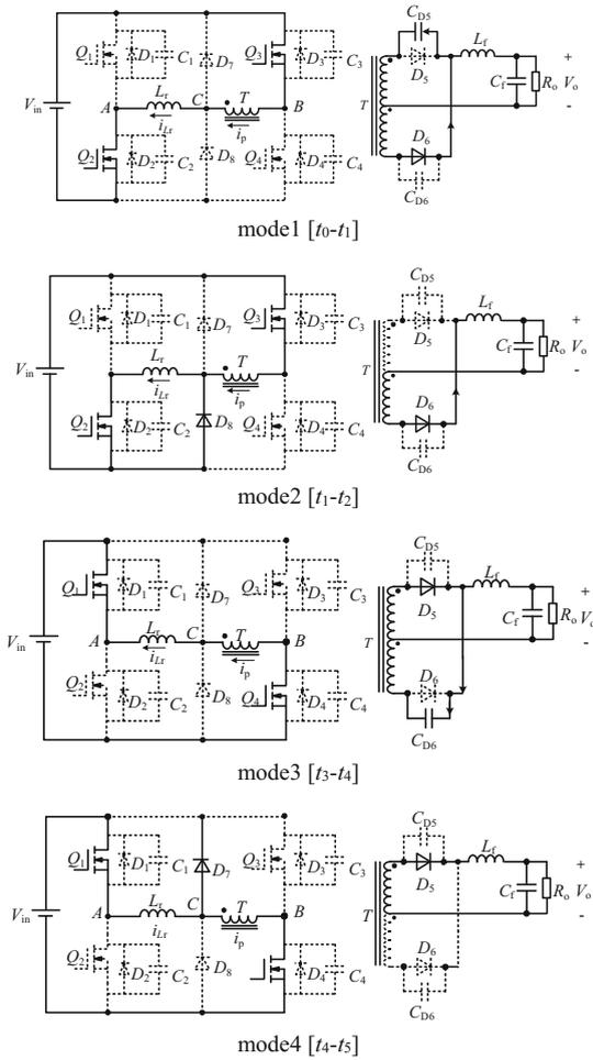
Fig. 4. Equivalent circuit diagram of clamping diode switching process
