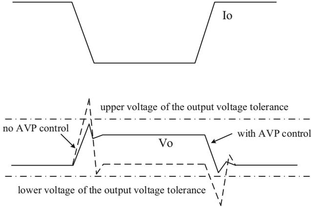
Fig. 1. Output current and output voltage of the converter with/without AVP control
