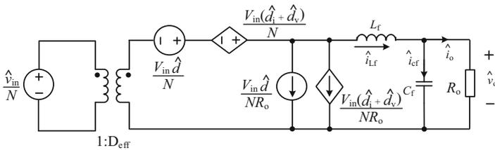
Fig. 7. Phase shifted full bridge soft switching small signal model
