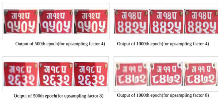
Fig. 4 Output of SRGAN model for up-sampling factor four and eight
