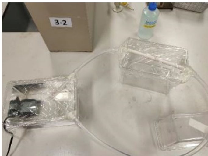
Fig. 52.2 Picture showing top view of the filtration set-up
