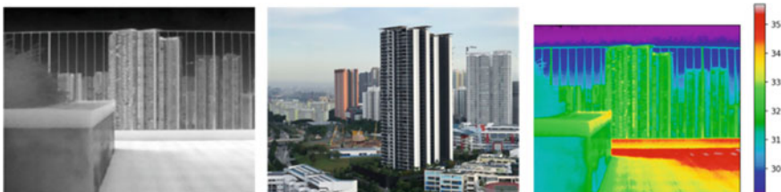
Fig. 13.1 Image on the left is captured by a thermal camera and the image on the right is captured by a conventional camera
