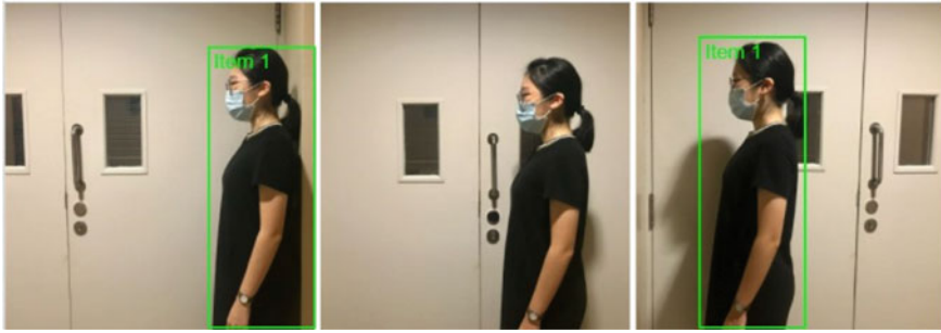
Fig. 42.5 Three consecutive output frames with failed detection in the second frame and successful detection in the first and third frame
