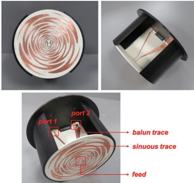
Fig. 27.10 Top and side views of antenna prototype, showing the sinuous trace and accompanying balun
