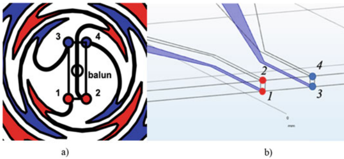
Fig. 27.9 a Top view of antenna feed and b connection points to balun
