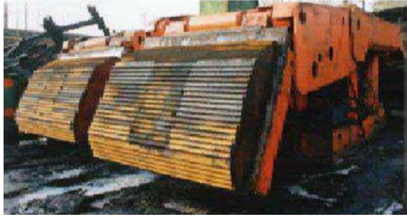
Fig. 9 Vibration system provided on the shield (Xie et al. 2006 cited by Alireza Jabinpour et al.)
