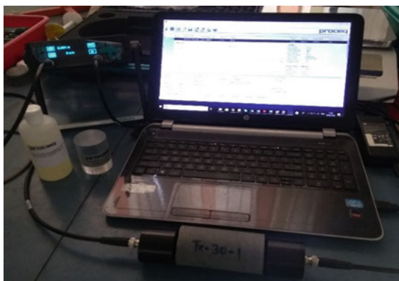
Fig. 2 P-wave PUNDIT instrument connected to a laptop and measuring the P-wave velocity of NX size specimens
