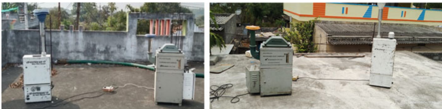
Fig. 2 PM_{10} and PM_{2.5} instruments placed in the nearby villages of the buffer zone
