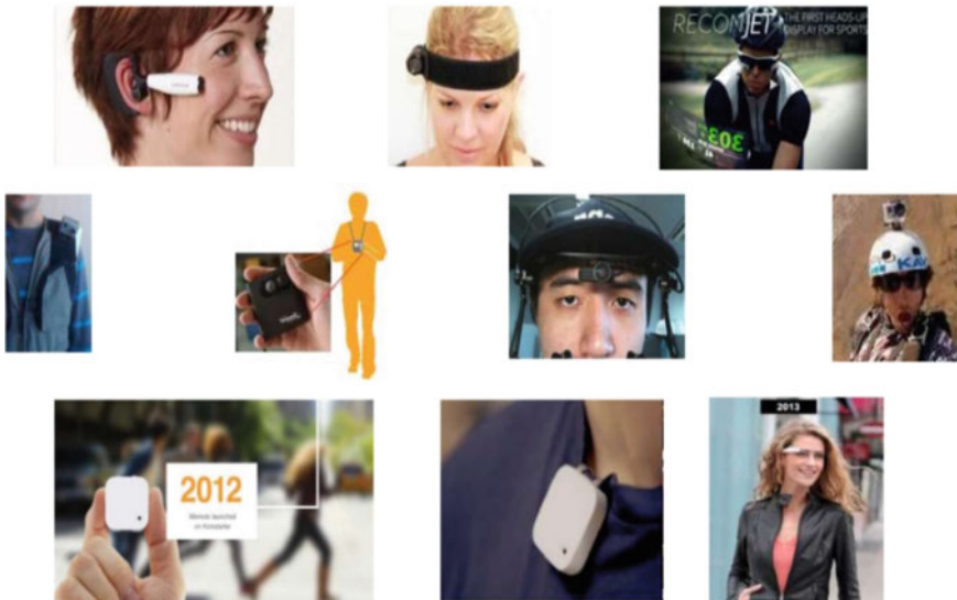
Fig. 2 Some common image sensor installation locations (Source Trung-Hieu Le thesis [17])
