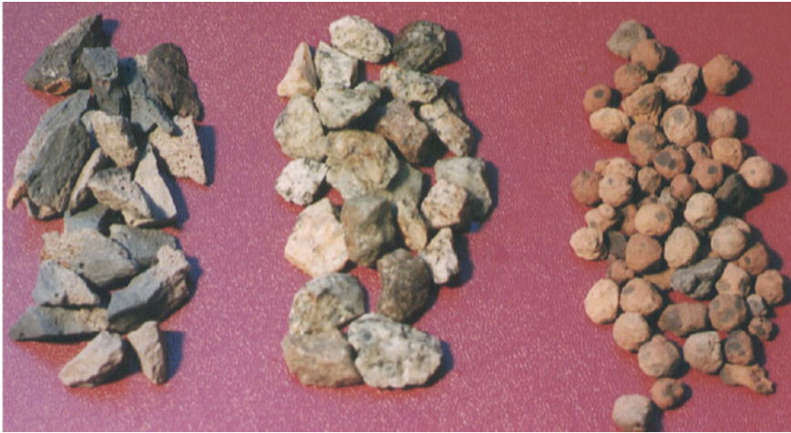
Fig. 17.2 Flashag (on the left), granite (in the middle), sintered fly ash aggregate (on the right) (Kayali 2005)
