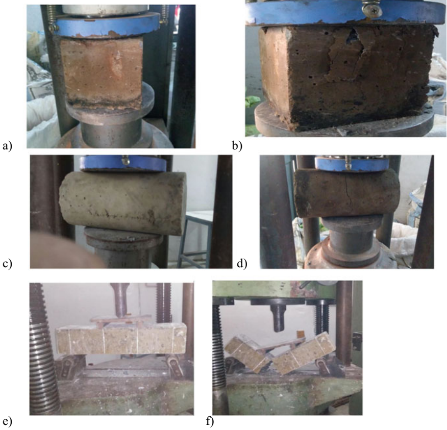
Fig. 14.2 Specimens of concrete for testing compressive strength, split tensile strength and flexural strength. a, c, e denotes before testing and b, d, f denotes after testing
