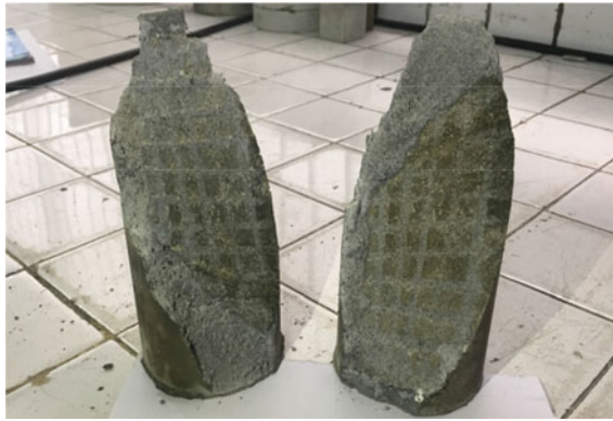
Fig. 19.3 Testing of bond strength by slant shear test as per ASTM C882
