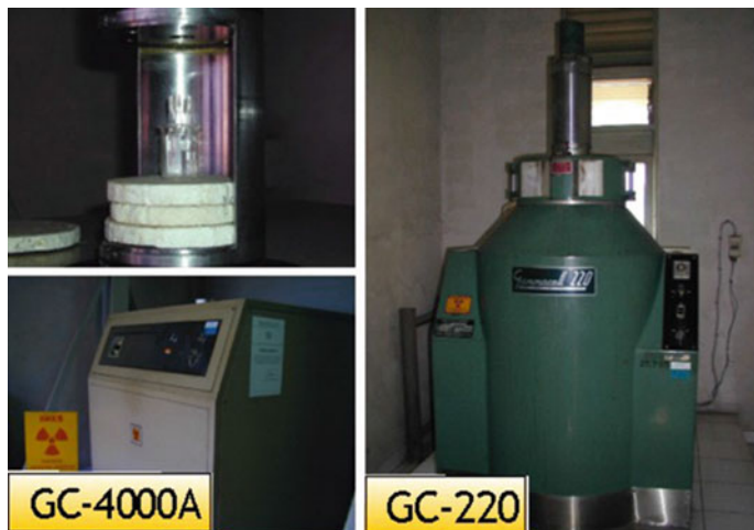
Fig. 14.1 Gamma irradiator with installed cobalt-60 source available at BATAN for irradiating breeding materials in mutation breeding program
