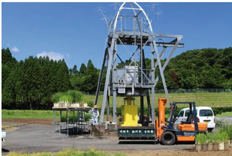
Fig. 12.17 A shelf between the ^{60}\text{Co} source of the irradiation tower and the nearest field, where the rice plants in pots were placed at ca. 5–3 m from the source in the Gamma Field. (Courtesy of IRB, NARO)
