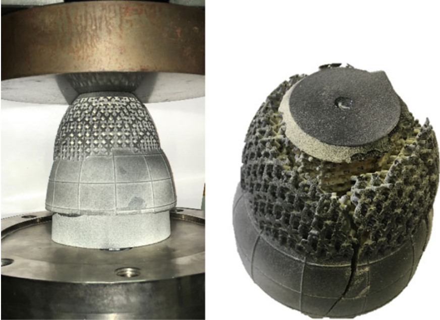
Fig. 7 Pressure test and break of the socket
