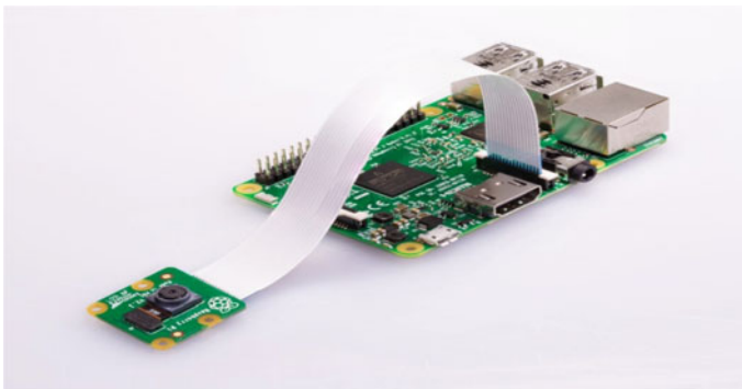
Fig. 3 Connecting Raspberry Pi cam with Raspberry Pi
