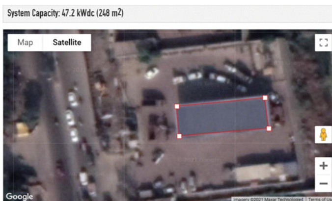
Fig. 1 The available rooftop area calculation using PVWatt web application version 6.1.4
