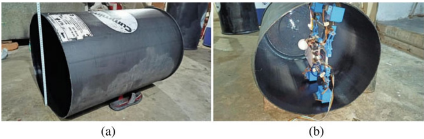
Fig. 5 a Oil drum-22 inches b Robot inside oil drum
