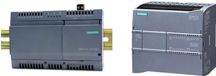
Fig. 4 a Siemens IOT2000 (left), b Siemens PLC s7200 (right)
