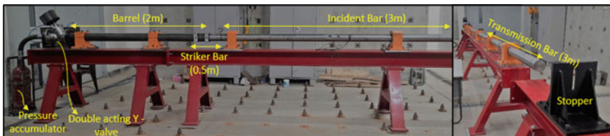
Fig. 5 Experimental test setup (SHPB)
