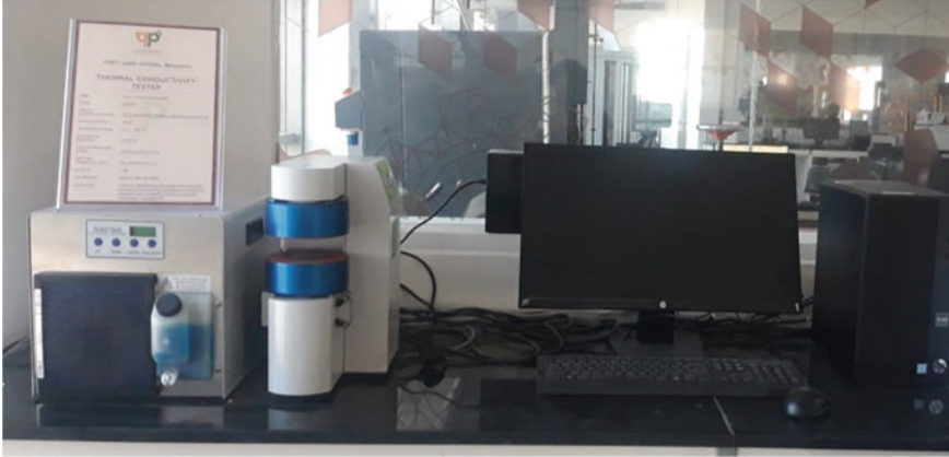
Fig. 2 FOX 50 heat flow metre experimental setup to measure thermal conductivity
