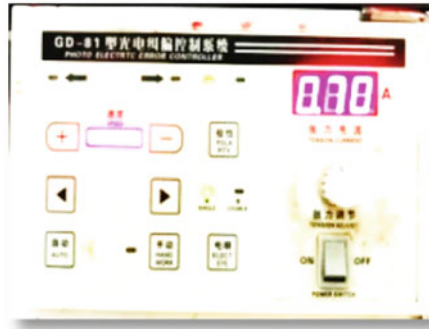
Fig. 6 Feed control unit
