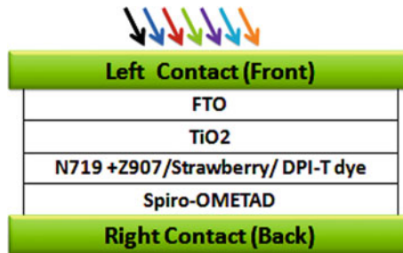
Fig. 2 The device structure of DSSC when using different dyes in SCAPS-1D
