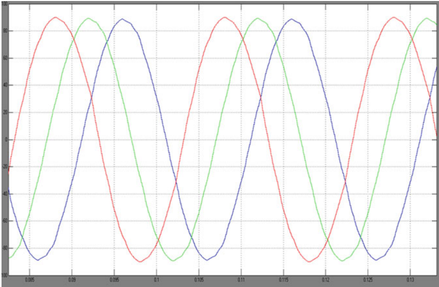
Fig. 13 Output voltage after compensation using SCMLI-based STATCOM
