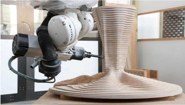
Fig. 15.1 Robotic milling of the Lily table using the Core Box tool bit. Credit Photography by LLDS
